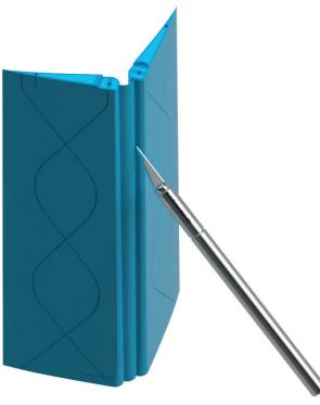
Black pins can be cut from 1mm carbon fiber rod, alternatively from 1mm steel rod.
